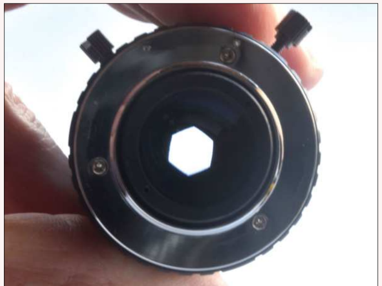
If you look through a lens while you adjust the aperture control, you'll clearly see the iris shutter open and close to increase or decrease the amount of light admitted to the camera.
