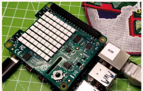
Designed for all 40-pin models of Raspberry Pi, Sense HAT is an old board that's still relevant in the classroom and space station!
