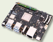
The VisionFive V1 is a single board PC based on a RISC-V processor.
